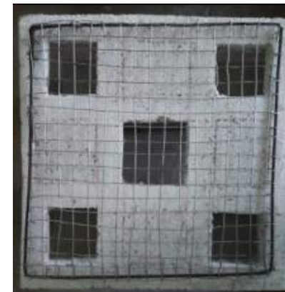
Perforated Ferrocement block
