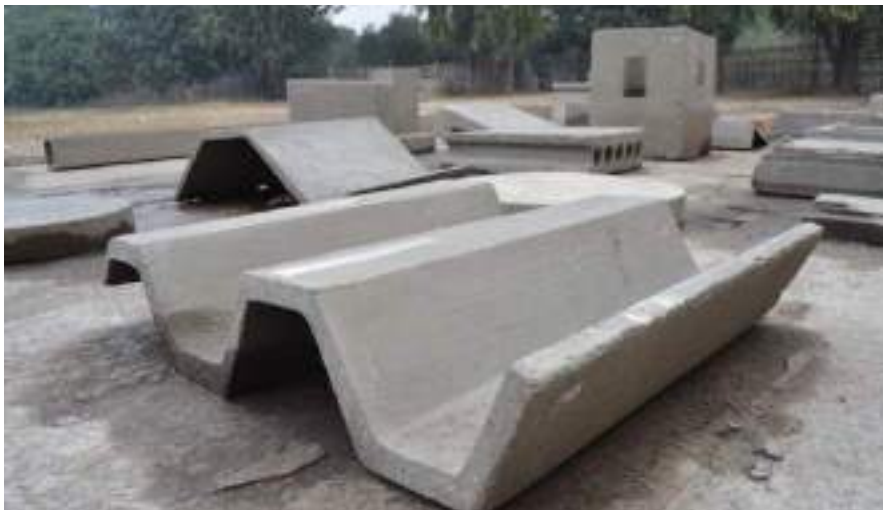
Ferrocement Folded Plate
