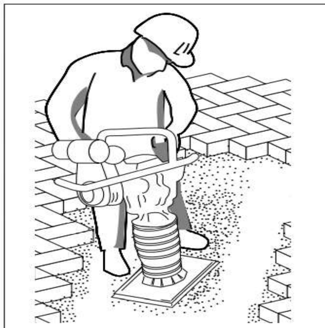
Figure 10. Compaction of the base in 2 to 4 in. (50 to 100 mm) lifts and monitoring density with a dynamic cone penetrometer or a nuclear density gauge are essential to minimizing settlement.
