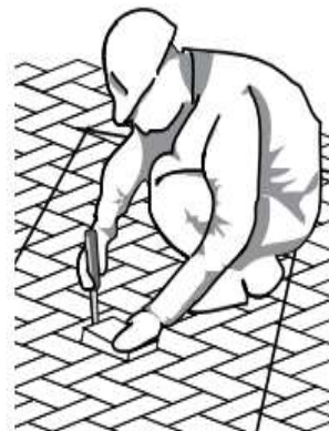
Figure 4. Prying with a screwdriver and pulling the paver out.
