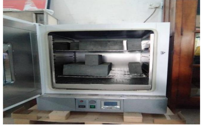
Oven curing at 90° C
